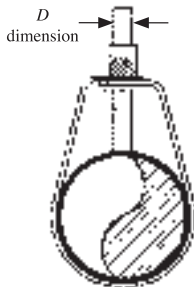
Adjustable swivel Ring - rod tight to pipe
